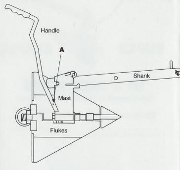
A Fit the handle to the position provided. (Relocate pin from Step 1A into handle).
