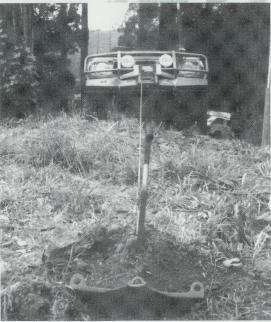
A ground anchor that's extremely compact and easy to use with a power winch or tirfor.
