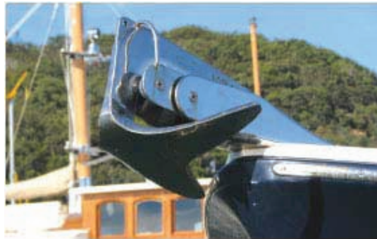
A very attractive stainless steel claw, Bruce type, anchor on a new motor launch. Low weight Claw/Bruce anchors will not set in some seabeds as they have blunt toes, and in this case too low a weight to penetrate.
