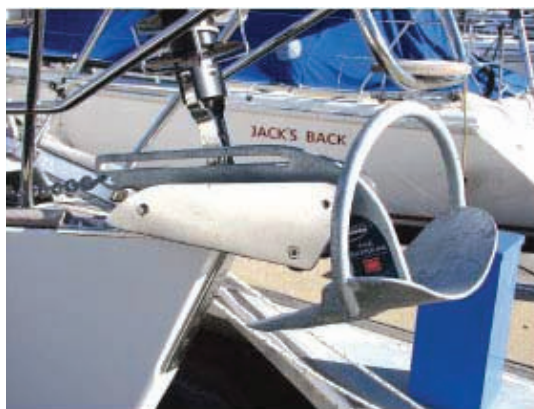
The Rocna and Manson Supreme anchors are almost identical. The Supreme has a slot to ease retrieval but ROCNA have introduced the same device on some of their models.
