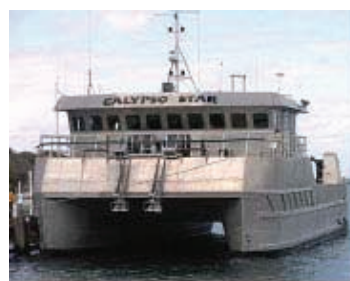
SARCA anchors are used on some serious work vessels, so do not think your yacht is too big. These 2 x 145kg anchors on the Calypso Star have been a complete success reducing downtime through dragging and recommended for similar vessels working the Bass Strait oilfields.
