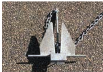
A typical Danforth copy, it looks like a Danforth but might differ, markedly, from the original design and has been sold with no specification. (Even $10 T-shirts declare the raw materials from which they are made) Danforth anchors are seldom seen on bow rollers as they can catch stray ropes.
