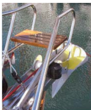
A Spade anchor on a Bulzen at the '07 Sydney Boat Show. The shank is bolted to the fluke which can be a weak point. These anchors have a very high reputation in Europe but are seldom seen in Australia.
