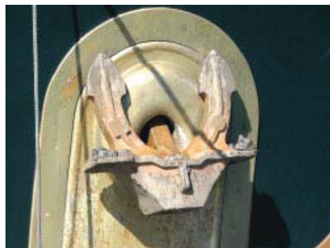
Cambria II carries 2 x 150kg Dreadnought type anchors and 2 x 150m of 5/8" chain. This is the only type of anchor that can be sensibly carried in a hawse pipe
