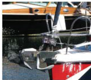
A Spade anchor on a yacht at the '07 Sydney Boat Show. The shank is bolted to the fluke which can be a weak point. These anchors have a very high reputation in Europe but are seldom seen in Australia.
