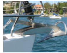
The German company Wasi introduced their Bugel anchor with a revolutionary roll bar to aid self righting. The original was only in stainless steel but was simple to copy and many galvanised versions exist. Very popular in Europe but almost unknown in Australia. This model is on a Beneteau.
